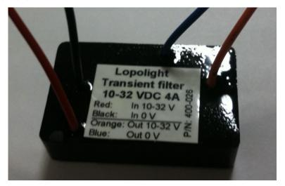
The Lopolight Transient Filter is to be fitted before any Lopolight (or other electrical device) on installations where heavy transients are expected.
